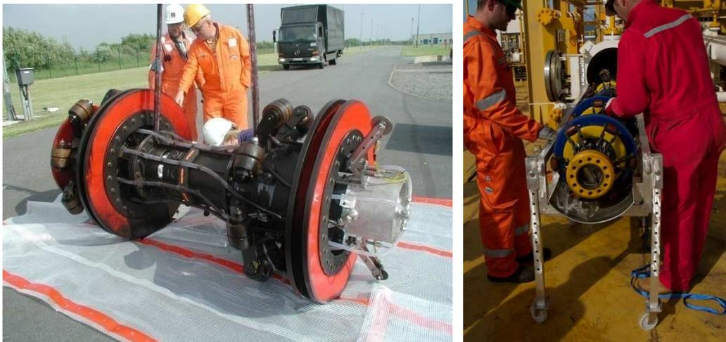
**Figure 47. Pipeline PIG.**
