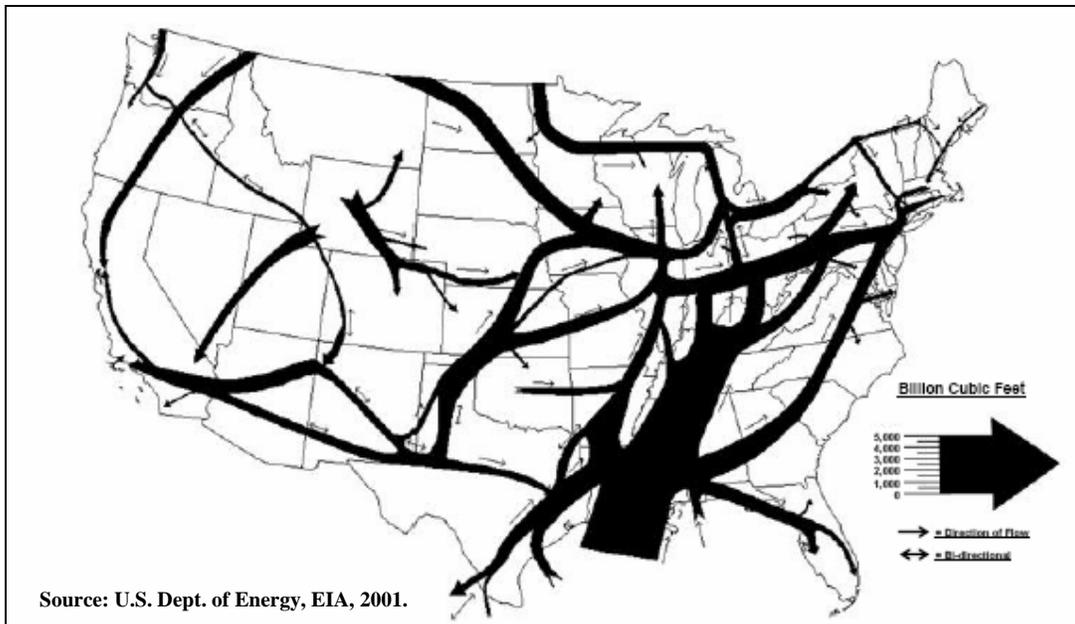
**Figure 50. Principle Interstate Natural Gas Flow Summary.**
