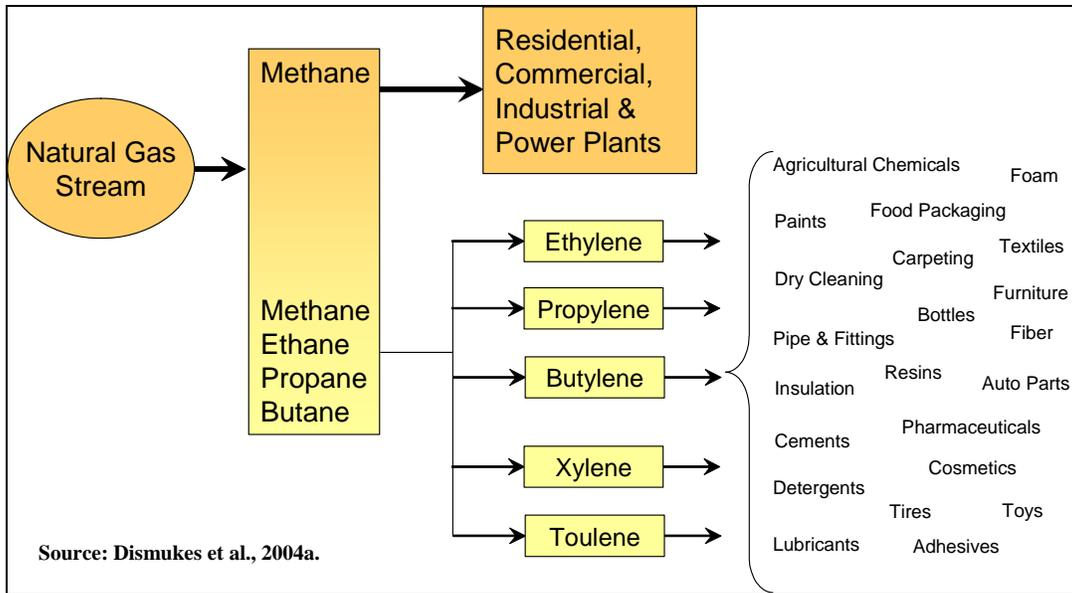
**Figure 14. Natural Gas Components and Petrochemical Products.**
