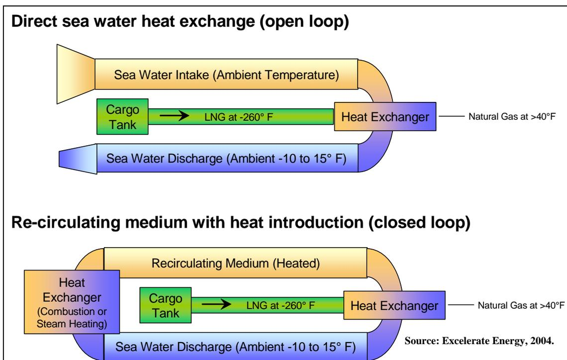
Figure 69. Primary Methods to Vaporize LNG.
