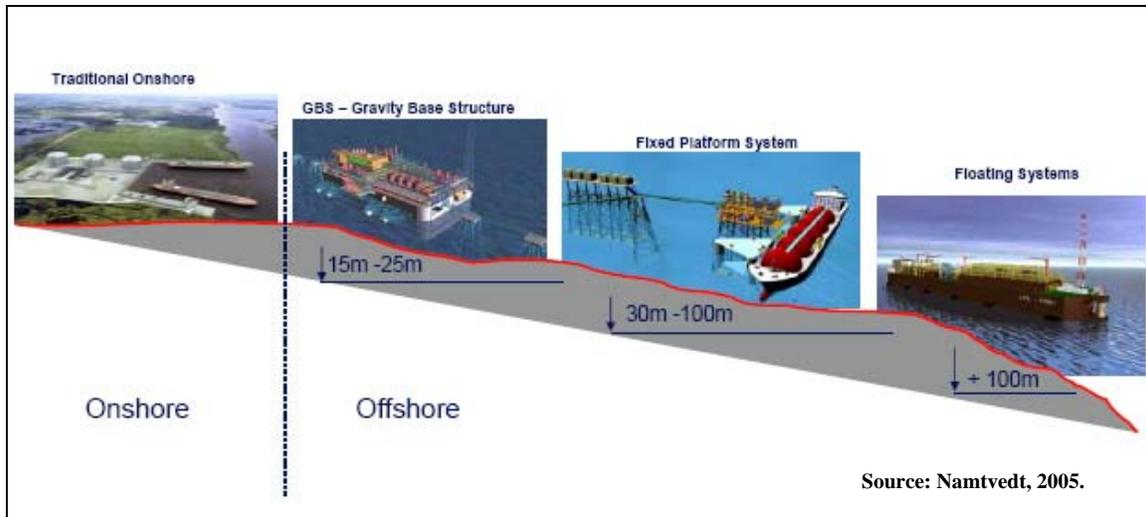
**Figure 39. Types and Locations of Typical Regasification Facilities.**
