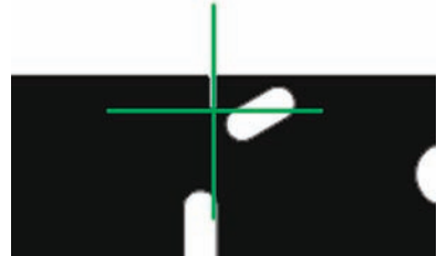
A single point is probed to measure the location of a point feature
