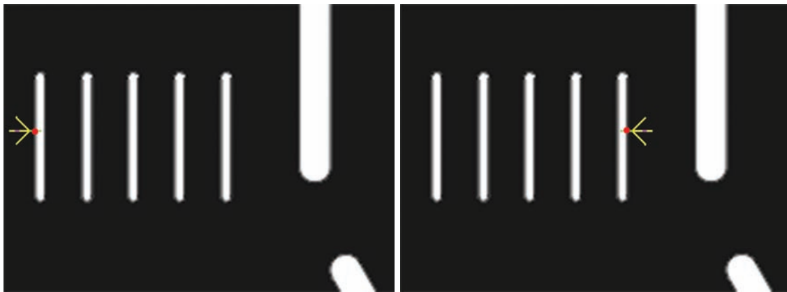
The distance across five slots is measured by probing two points using the Simple probe
