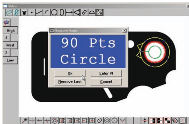
Ninety points are probed using the Circle probe to measure a circle feature
