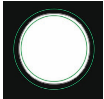
Video chart for the visual inspection of a hole
