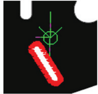
Scans are completed around the perimeter of the feature
