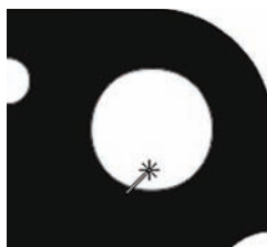
A circle measurement is performed using the circle probe
