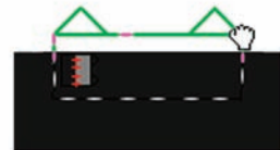
the second point is dragged across the edge to create a Buffer probe
